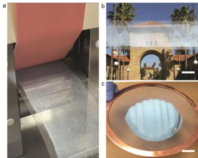
Figure 4. (a) Photograph of a roll-to-roll process to transfer electrospun nanofiber film onto plastic mesh. (b) Photograph of a roll-to-roll produced transparent air filter. The scale bar is 5 cm. (c) Photograph showing that freestanding nanofiber film can be easily transferred onto a facemask. The scale bar is 3 cm.
